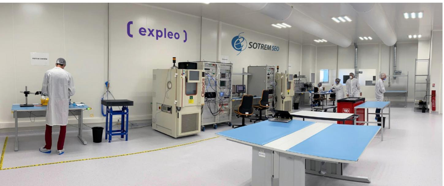
Our ISO 8-compliant clean room in Toulouse, France provides a secure environment for the testing and tuning of space equipment, such as subsystems for nanosatellites. The highly monitored facility also offers valuable storage space, as well as a platform for our space team to expand our engineering and testing services.
